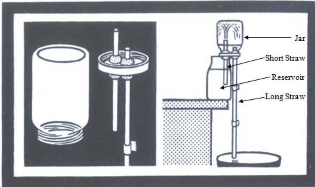
Figure 1: Sketch of a miniature water fountain built and used as a testing apparatus [18].
