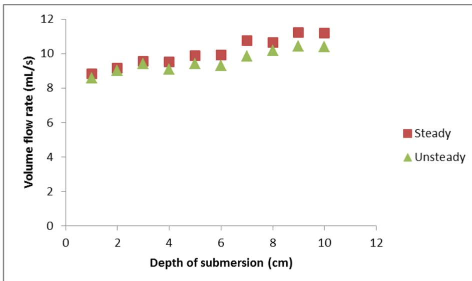
Figure 4: Depth of submersion versus flow rate for steady and unsteady flow.
