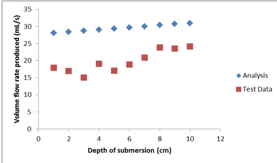
Figure 3: Volume flow rates in steady flow versus depth of submersion of the intake straw.
